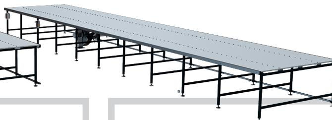
*Blowing table tops are properly drilled for the passage of air and they are supplied with motor and electric control panel every section of length.*
